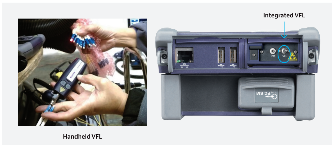
Figure 2: Fiber continuity test
