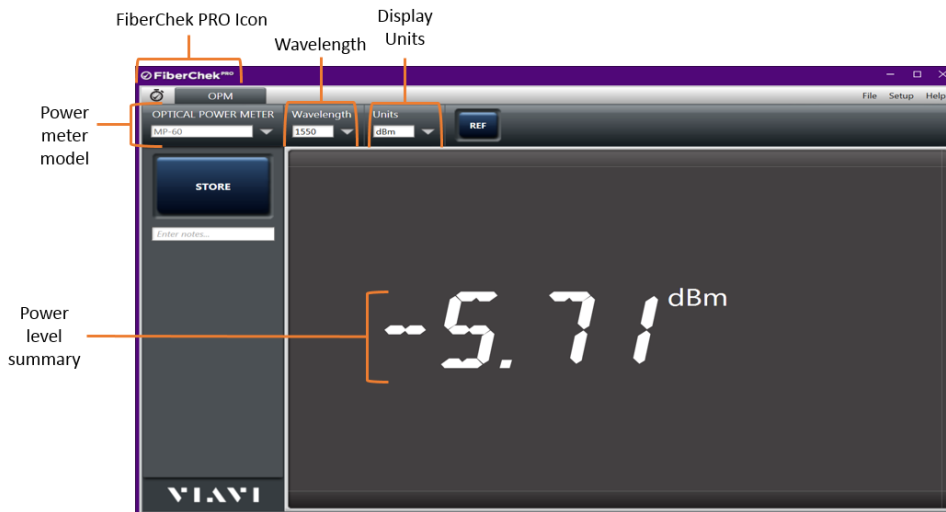
Figure 3: FiberChek PRO Power Meter View
