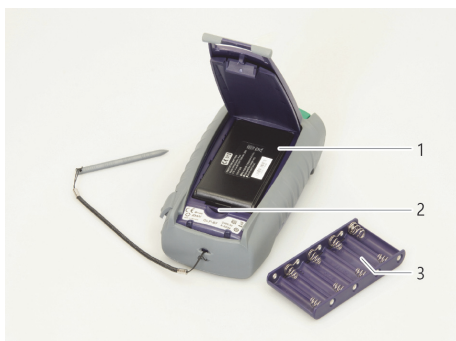
Fig. 5 Replacing the batteries
