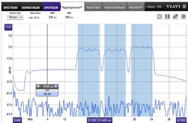
Figure 10. VSE-1100 HyperSpectrum display with live and max trace with DOCSIS and impulse noise
