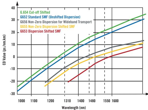
Figure 2: Expected CD values based on fiber type
