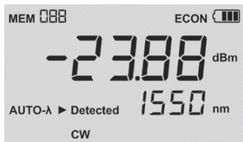
Fig. 5 Display in Auto- \lambda mode showing one detected wavelength and its power levels.
