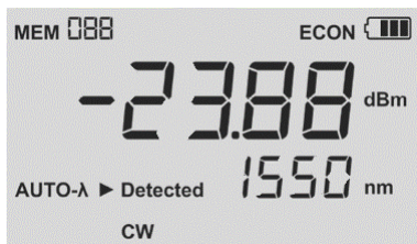
Fig. 4 Displaying absolute power level in dBm.
