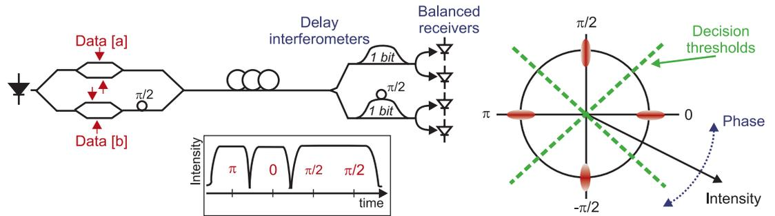
Figure 3: DQPSK - differential quadrature phase shift keying/differential detection
