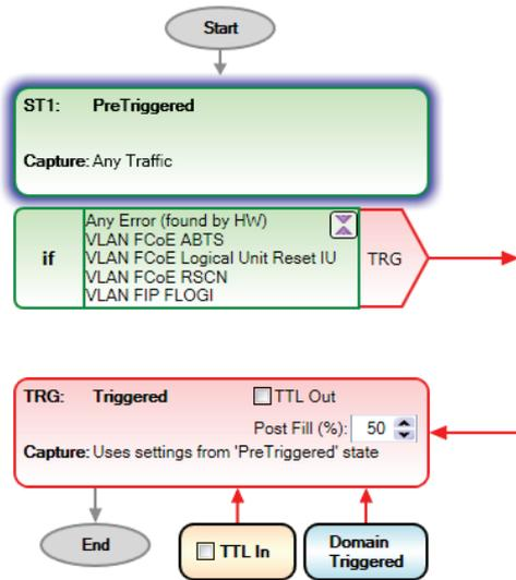
Figure 4. TraceControl trigger/filter configuration
