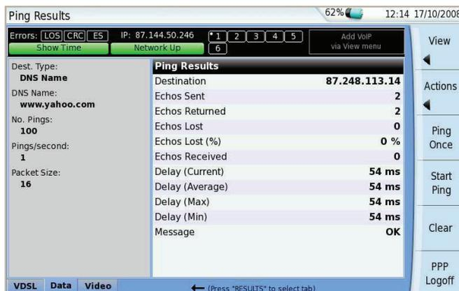
Figure 7. IP Ping test interface
