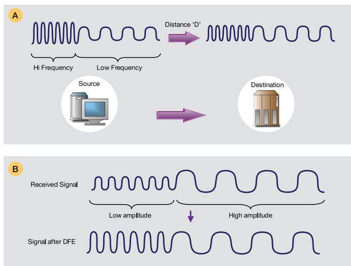
Gb/s SAS-2 overcomes attenuation effects by de-emphasizing lower frequency components at the transmitter as well as by selectively boosting higher frequency components on the receive side (see Figure 2B) using an equalization method called Decision Feedback Equalization (DFE). Developers designing or troubleshooting SATA Gen-3 equipment must resolve attenuation and jitter issues differently as SATA Gen-3 does not support either de-emphasis or equalization.
