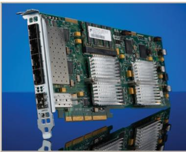
Figure 7. J6872A 10 Gigabit/Gigabit Ethernet high-performance interface card
