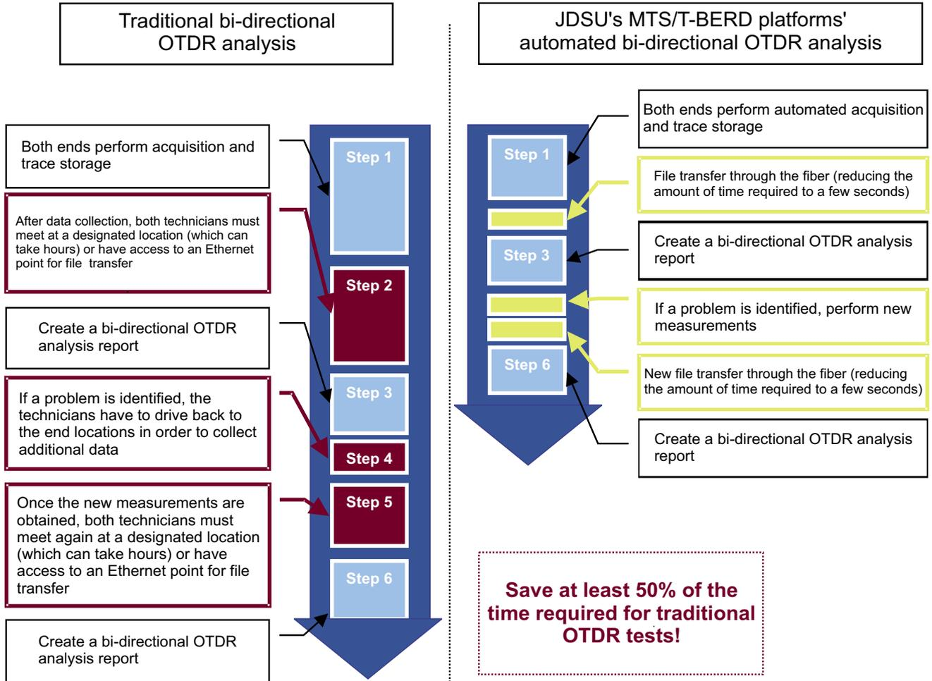
**Installer test: JDSU's automated bi-directional OTDR analysis for 72 fibers at 2 wavelengths: 2 hours**
