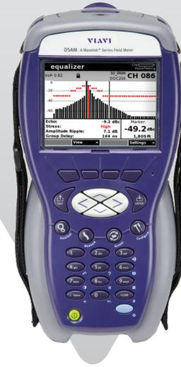
The DSAM Equalizer Option speeds downstream troubleshooting and helps uncover hidden faults by providing enhanced quadrature-amplitude modulation (QAM) signal information. The equalizer mode graphs the DOCSIS receiver equalizer taps so technicians can identify problem-causing reflections quickly.
