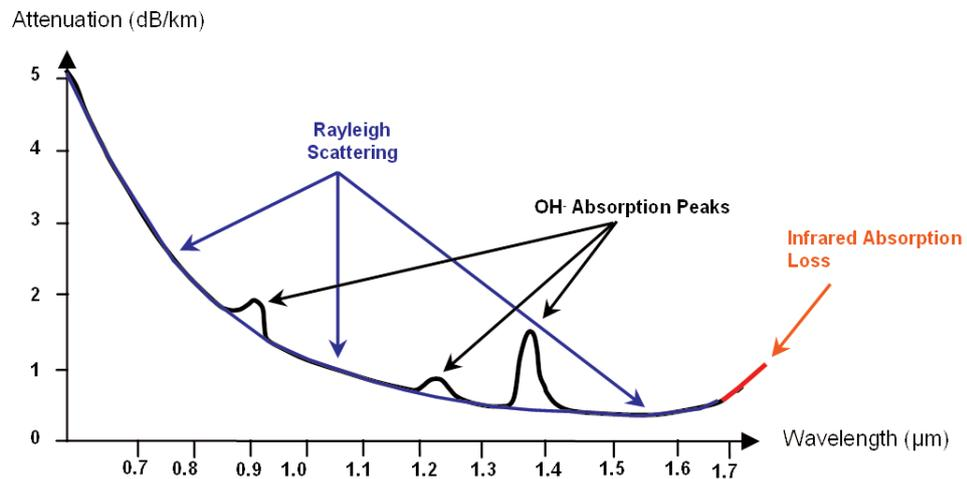
Figure 2. Relationship between wavelength and total fiber attenuation
