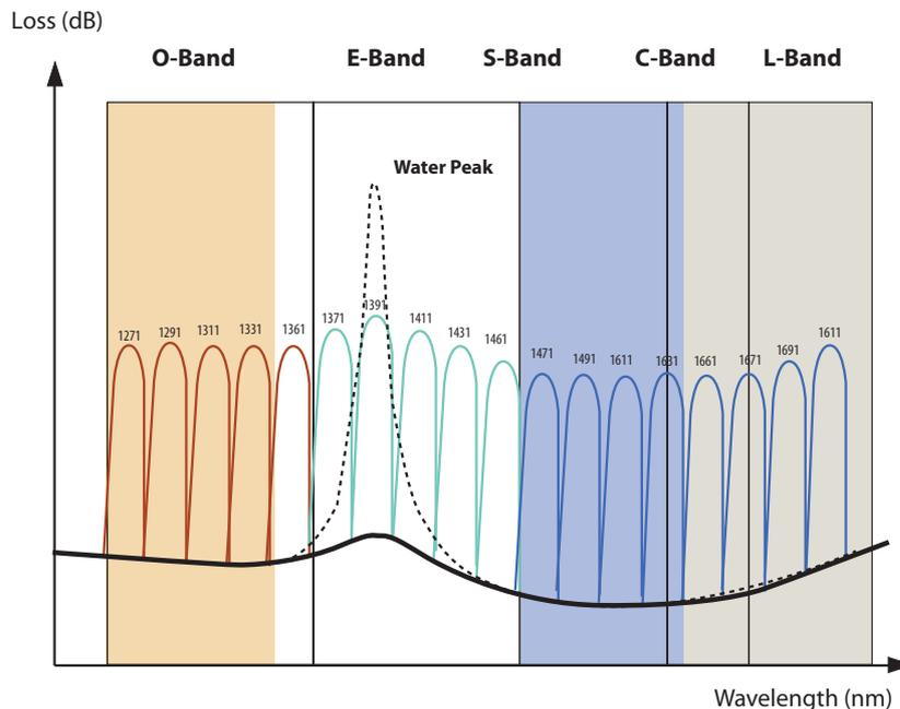
Figure 1. CWDM wavelength allocation and fiber loss
