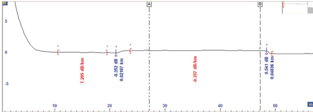
Figure 2. OTDR display of a section of fiber with an elevated K coefficient
