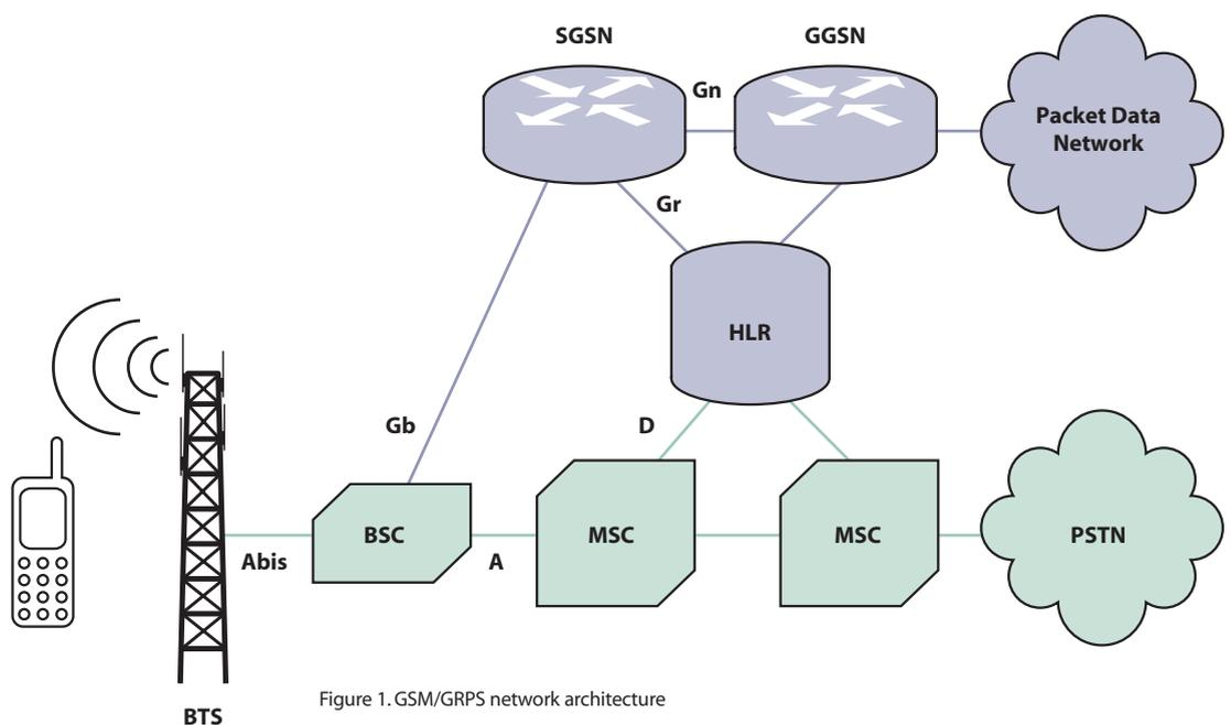
Figure 1. GSM/GRPS network architecture
