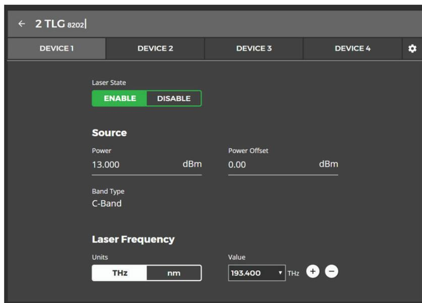
Figure 2 – mTLG MAP-300 detailed view GUI
