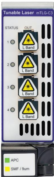
The mTLG-C3 is based on a Sampled Grating Distributed Bragg Reflector (SG-DBR) laser with an integral wavelength locker. Wavelength and output power settings can be controlled using the MAP series local interface or automation interfaces. The integrated wavelength locker and automatic power control loop provide stable operation. The mTLG-C3 module is a new generation tunable laser module, which is ideal for DWDM testing where the capability to change.
