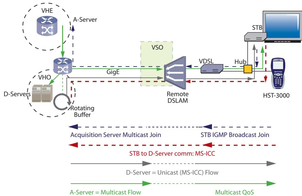
Figure 1. STP initiating the IGMP join message as well as the ICC Protocol message
