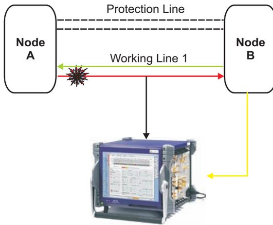
Figure 14: An interoperability test to determine the line side to client side detection and response time
