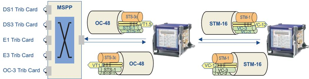
Figure 4: Example test setup using ONT multi-channel test solution.
