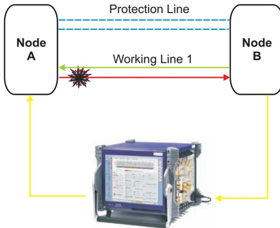
Figure 15: A network test to determine service disruption time.
