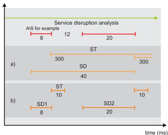
Figure 10: An example of one service disruption scenario measured with two different separation time settings.
