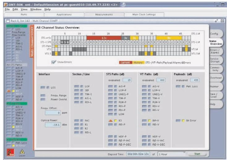
Figure 5. The All Channel Status Overview provides error/alarm information in real-time for all channels under test at a glance.
