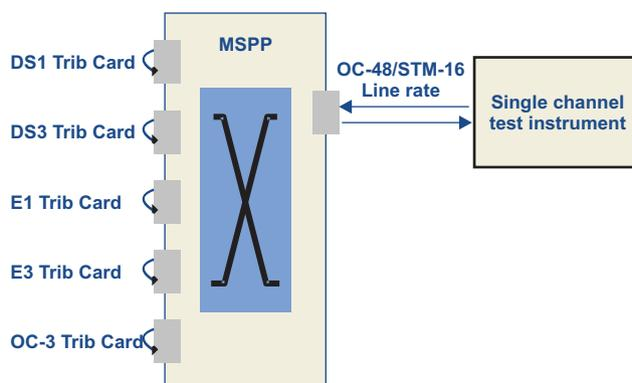
Figure 3: Example test setup using traditional single channel test instrument.
