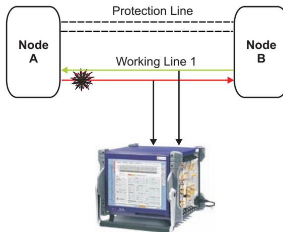
Figure 13: An interoperability network test to determine the line side error/alarm detection and K1/K2 command response time.
