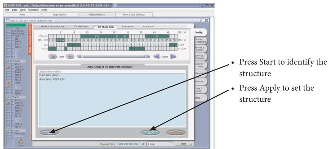
Figure 6: The Auto-Setup function identifies complex signal structures, overhead, section and path traces, and payloads in a matter of seconds.
