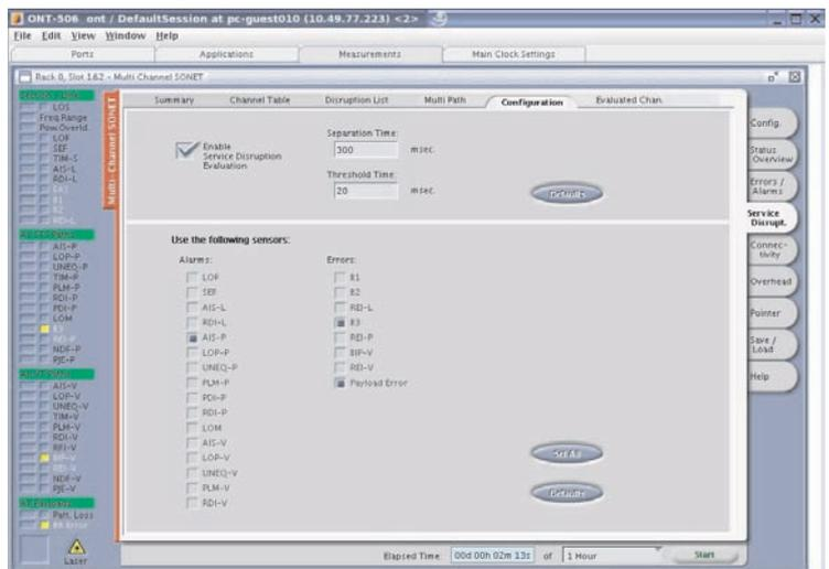
Figure 9: Flexible trigger criteria allow for full customization of service disruption measurements.
