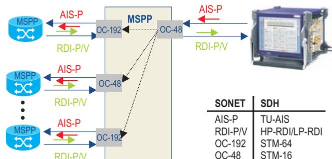
Figure 7: Error and alarm “flooding” of the network (SONET example).
