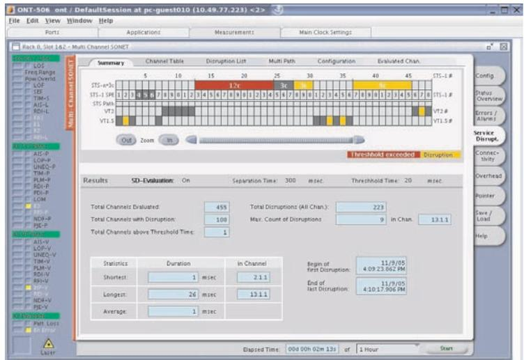
Figure 8: Overview and status of all channels under test and real-time display of Shortest, Longest and Last service disruption measurements.
