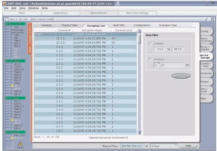
Figure 11: Service disruption list of all channels under test.
