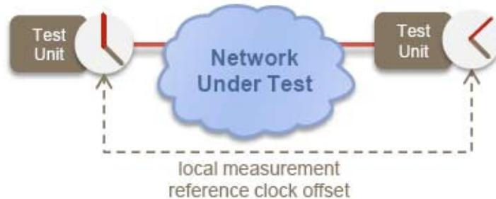
Reference Clock Sync Required for 1-Way Measurements
