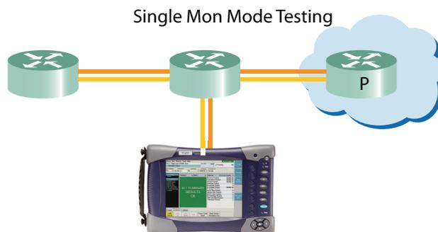
Figure 10. T-BERD/MTS-6000A monitors traffic forwarded by a router/switch mirror port or network tap
