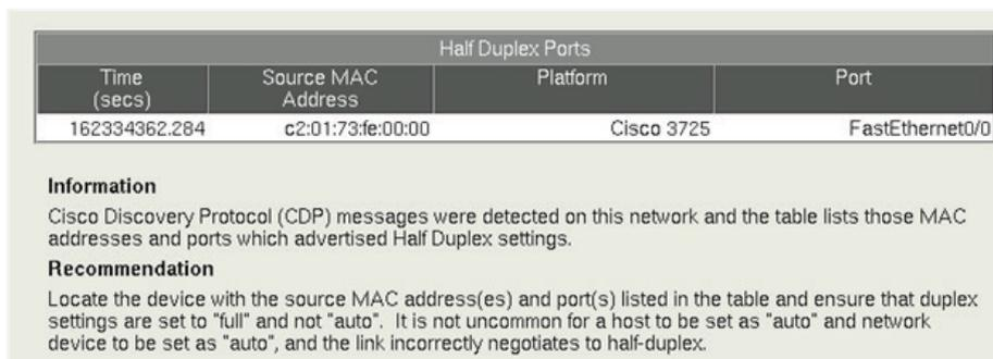
Figure 5. J-Mentor Half-Duplex Testing Results
