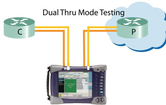
Figure 11. The T-BERD/MTS-6000A testing in dual Through Mode
