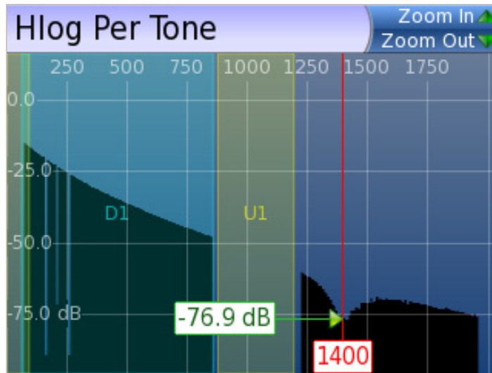
Figure 2. A bridged tap caused a "dip" on the Hlog frequency response curve. The example shows a bridged tap length of approximately 8 m.
