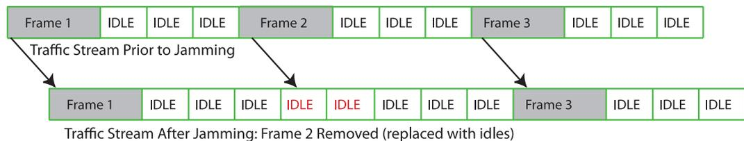
Figure 3: A “Disappearing” Frame (Replaced by Idles)
