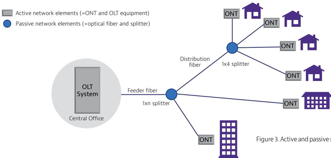
Figure 3. Active and passive network elements
