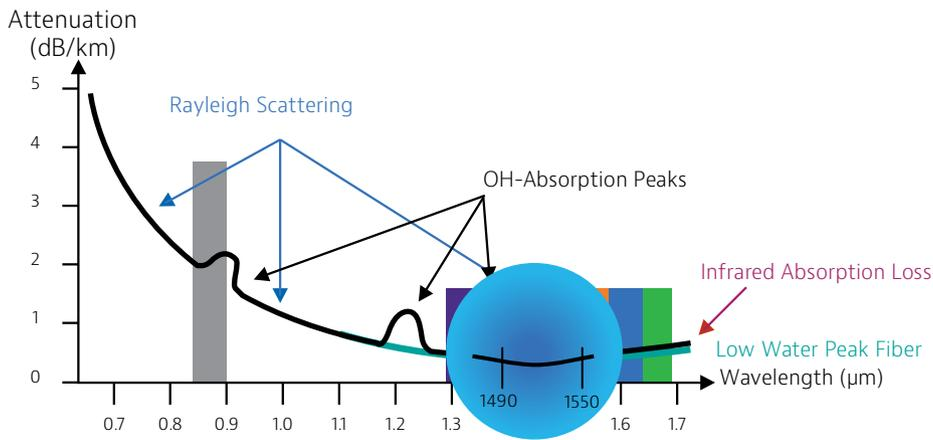
Even if some fiber manufacturers give a specification at 1490 nm the example table below demonstrates that measuring insertion loss at 1490 and 1550 nm gives very close results.
