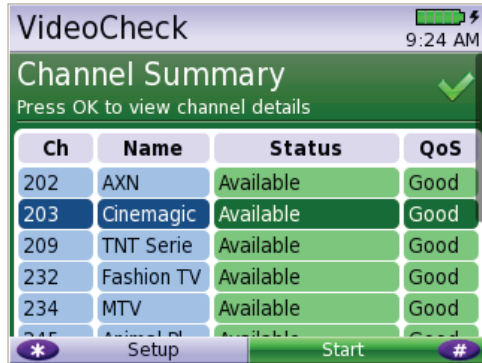
Figure 3. The SmartClass TPS VideoCheck channel summary shows each channel's availability as well as the QoS.
