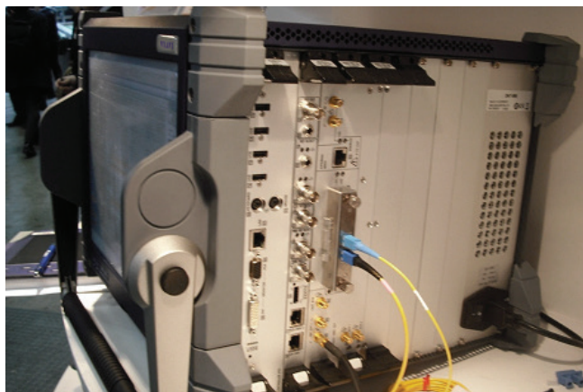
Figure 5. CFP LR4 module inserted in ONT tester
