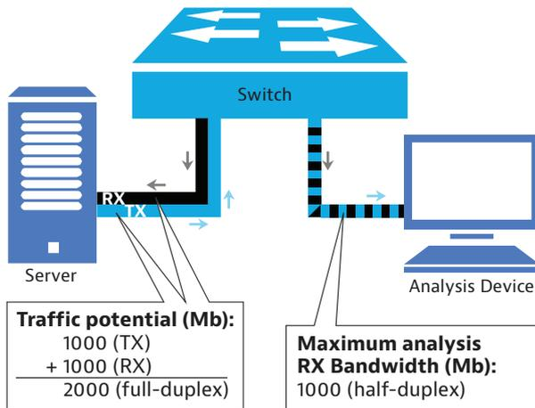
**A TAP delivers both TX and RX signals, separately** providing a pass-through signal for network traffic, and a full-duplex, line-rate signal to a monitoring device.
