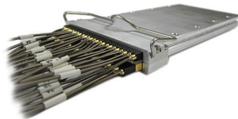
Figure 7. The CFP electrical adapter maintains electrical access to all high-speed CAUI/XLAUI signals
