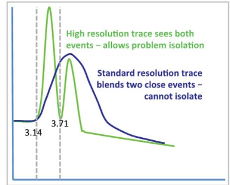
Figure 5. Resolution comparison standard-res OTDR to EVO-A
