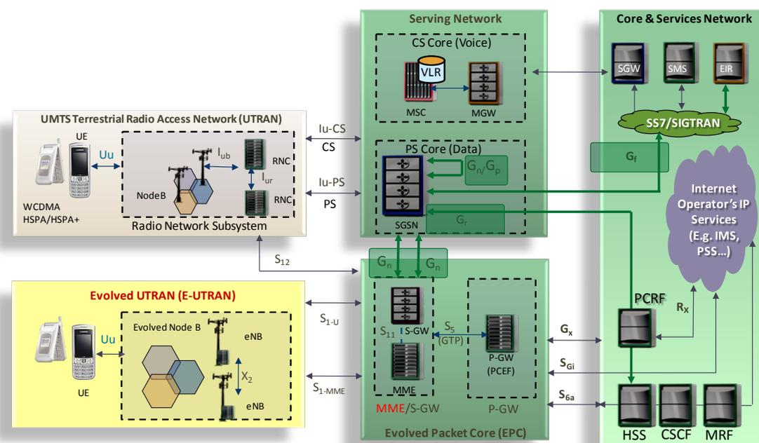
Figure 2. Control functions of the RNC have moved into the eNodeB
