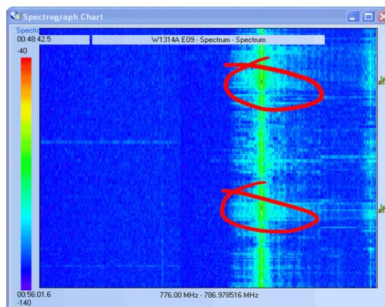
Figure 4. Drive test spectrograph for identifying interfering signals
