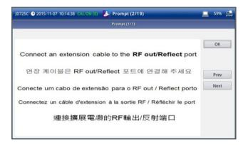
5. Perform electronic calibration using the EZ-Cal kit.
