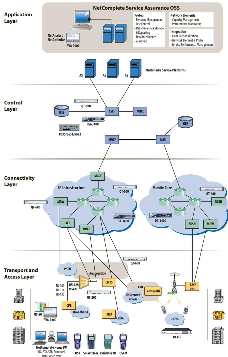
Figure 8 JDSU can provide complete service assurance coverage over an FMC service
