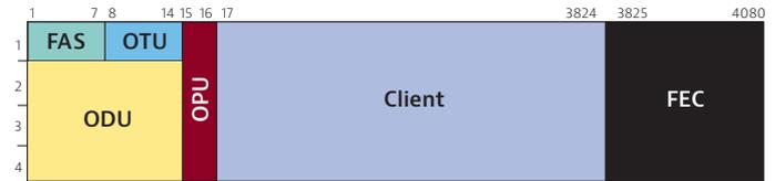
Figure 6: Optical channel structure consisting of OH bytes, client, and FEC
