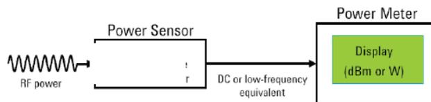
This above diagram shows the basic methodology of measuring high frequency power using the combination of power meter and power sensor. The power sensor converts high frequency power to a DC or low frequency signal that the power measure can measure and relate to an RF power level. The meter displays the direct signal as a power value in decibels or watts.
