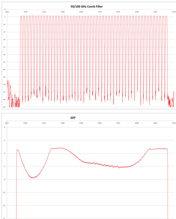
Figure 7. Examples of full span shapes: a comb filter (top) and gain flattening filter (bottom)
