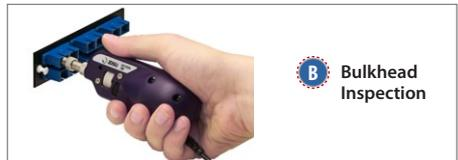
1. Select the connector you are testing and disconnect from the system.
