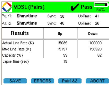
Bonded test results can be viewed as an aggregate or individually
