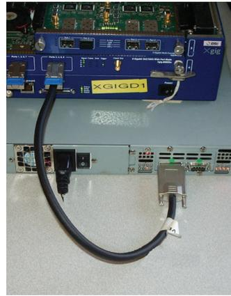
Appropriate Test Setup: 1) Signals are sent over a single cable, 2) the cable is a minimum length (short), and 3) the cable is properly shielded and rated for 6 Gb/s use.
