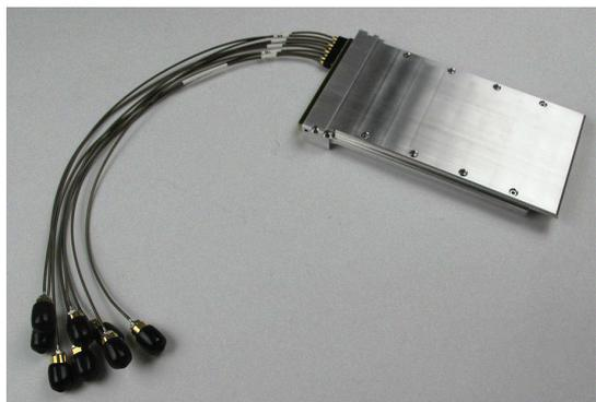
Figure 2. Electrical CFP adapter with partial cable set connected
