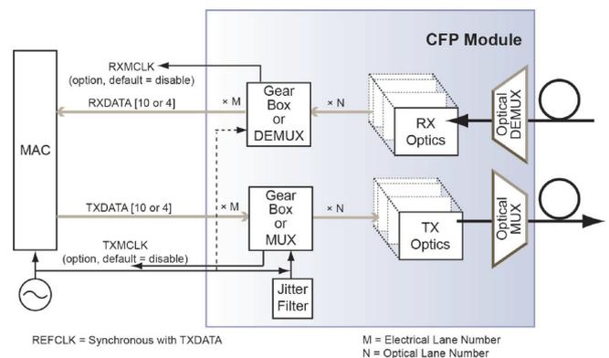
Figure 1. Typical 100G CFP block diagram
