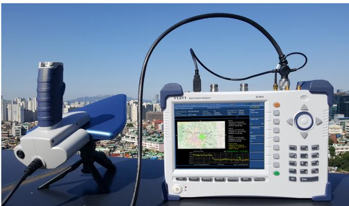
To meet trial deadlines, the Viavi NEM partner was not able to remove the source of interference. Instead, they used CellAdvisor measurements to relocate the radio head. Consequent measurements indicated a reduced level of interference near the new location. The radio was brought back in service. This let our NEM partner complete their customer proof-of-concept in a timely manner.
