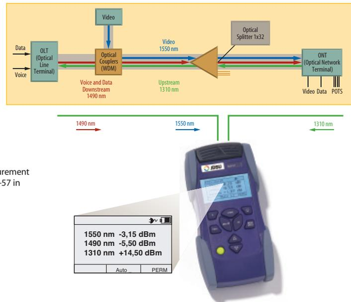
Figure 2 Selective level measurement in PON networks with the OLP-57 in Through Mode
