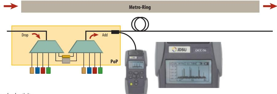
Figure 6 Channel loss and selectivity of CWDM multiplexers with the MTS-8000
