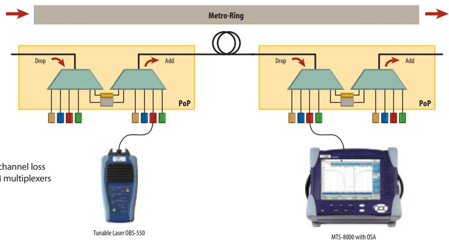
Figure 5 Test setup for channel loss and selectivity of CWDM multiplexers with the MTS-8000
