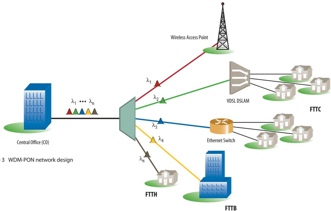
Figure 3 WDM-PON network design
