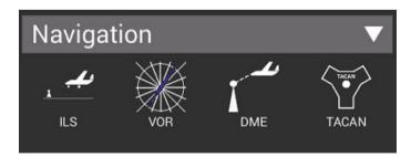
**ILS** — Provides simultaneous Localizer (with swept DDM), Glideslope and Marker Beacon Signals.
