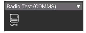
**COMM AM** — Provides signal generation over the Range of 10.00 to 400.00 MHz in 1 kHz increments and monitoring of transmitter power and modulation depth over the same range. A calibrated 1020 Hz tone, amplitude modulated at 30%, is also provided. Frequency control is provided in 8.33 kHz / 25 kHz channel steps or in 1 kHz variable steps. Audio output is available.
