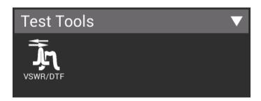
**VSWR / DTF** — This test tool is provided to assist in troubleshooting RF level issues. Test mode for both VSWR and Distance To Fault (DTF) testing can be set to VSWR or Return Loss.
