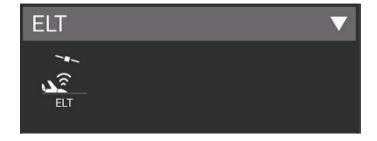
**121.5/243 BCN Modes** — Provides monitoring for 121.5/243 MHz swept tone short range Beacons and displays transmitter frequency, power and start/stop tone frequencies. Audio output is available.
