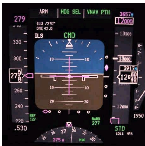
EFIS with 2 1/2 Dot ILS Deviation Figure 4
