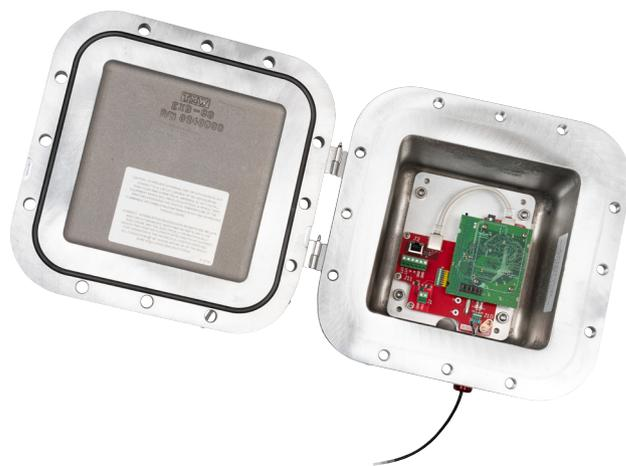
Figure 2. MicroNIR PAT-Lx barrier box interior. Ethernet, power, and trigger connect at the main circuit board through three dedicated ports, using HazLoc-rated connections.
