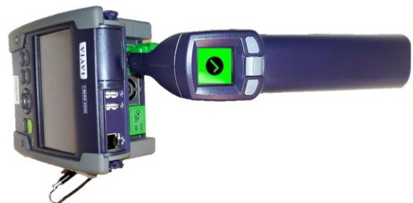
Figure 3: OTDR Port Inspection
