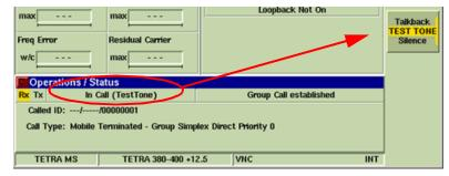
Fig. 5-43 Audio Test - Test Tone Selected
