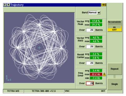
Fig. 5-9 TETRA MS Trajectory Tile - Maximized View
