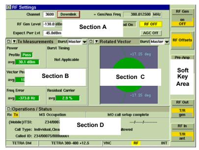
Fig. 9-1 TETRA DM System Display - Minimized Tiles
