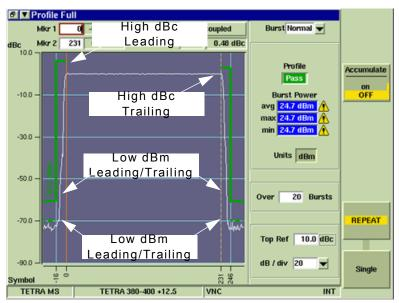
Fig. 4-24 TETRA MS Power Profile Full Tile - Limit Points Shown
