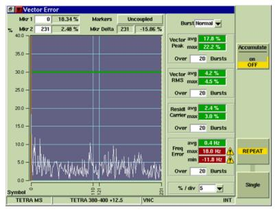
Fig. 5-10 TETRA MS Vector Error Tile - Maximized View
