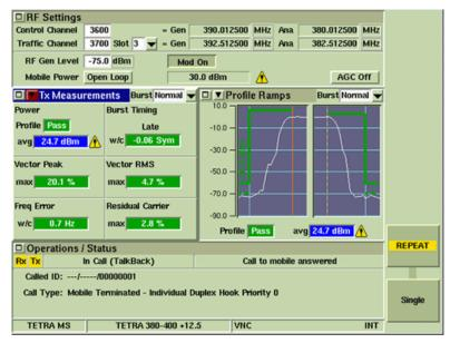
Fig. 5-27 TETRA MS Tx Measurement Tile - Minimized View
