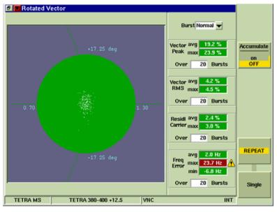
Fig. 4-26 TETRA MS Rotated Vector Tile - Peak Limit Shown
