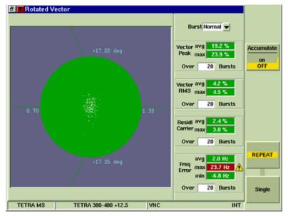
Fig. 5-8 TETRA MS Rotated Vector Tile - Maximized View
