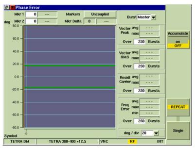
Fig. 9-18 TETRA DM Phase Error Tile - Maximized View
