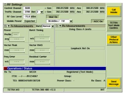
Fig. 5-12 TETRA MS Operations/Status Tile - TT Test Mode Registration
