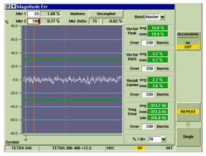
Fig. 9-17 TETRA DM Magnitude Error Tile - Maximized View
