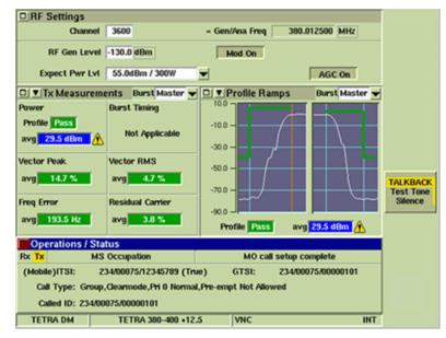
Fig. 9-22 TETRA DM Operations/Status Tile - Minimized View
