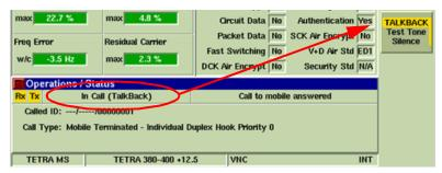
Fig. 5-42 Audio Test - Talkback Mode Selected
