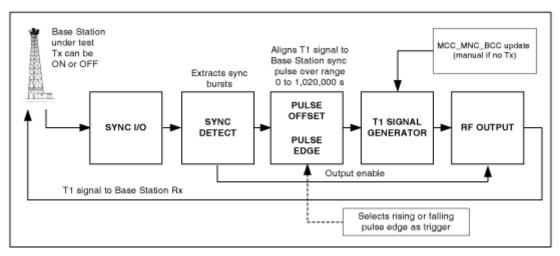
PULSE MODE Fig. 8-2 Diagram of Sync to Base Station - Auto and Pulse Modes
