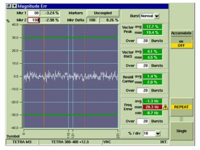
Fig. 5-6 TETRA MS Magnitude Error Tile - Maximized View
