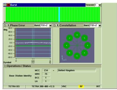
Fig. 7-3 TETRA BS Burst Tile - RF Settings Tile location
