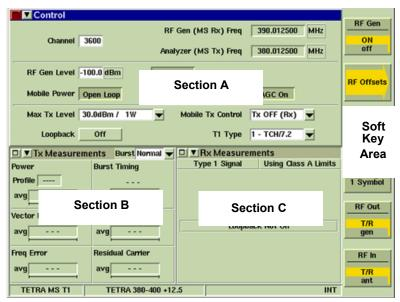
Fig. 6-1 TETRA MS T1 System Display - Minimized View
