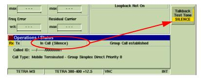
Fig. 5-44 Audio Test - Silence Mode Selected
