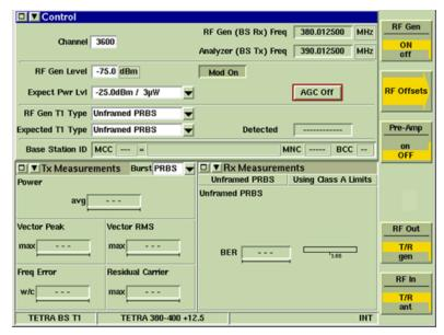
Fig. 8-5 TETRA BS T1 Control Tile - Channel Plan Selected
