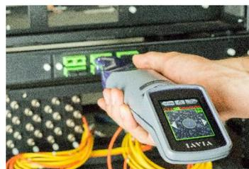
Figure 9: Bulkhead connector
