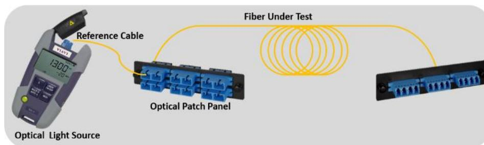
Figure 1: Connecting OLS to OPP or coupler
