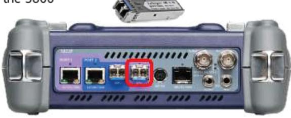
2. Inspect the SFP with the fiber microscope and a bulkhead tip
