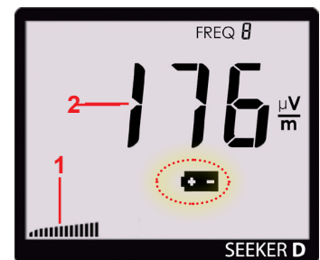
Battery Charge Level
