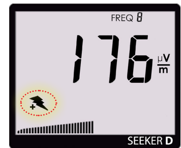
Battery Charging Status
