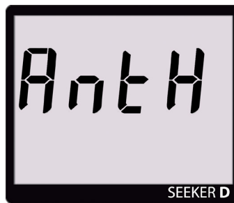
Attach High Band Antenna
